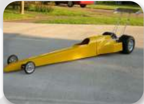
The Vaporzor top fuel dragster was one of the early dragster models offered by Pacesetter. It was chain driven and had a full body.
