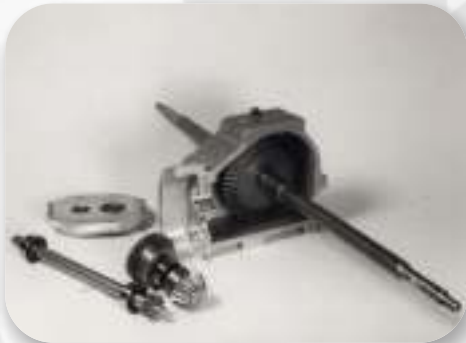
Not only was Pacesetter the first to develop a 1/4 scale car in the US, they were the first to develop a Quick Change rear end that was included in almost ALL their 60's style sprint cars.
